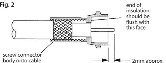
The inner wire of the cable should protrude about 2 mm beyond the nut end of the plug.
