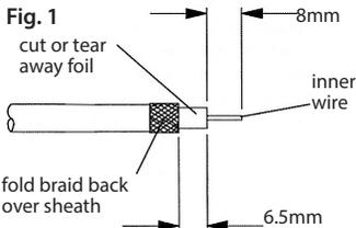
Measure cable run first and cut cable to fit with a bit to spare. Slide one of the weather boots provided over the aerial end of the cable. Prepare both ends of the cable as shown in Fig. 1. Fold the braid wires of the cable back over the sheath and fit one of the screw-on type-F plugs.
