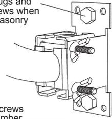
use the wood screws when fixing to timber
